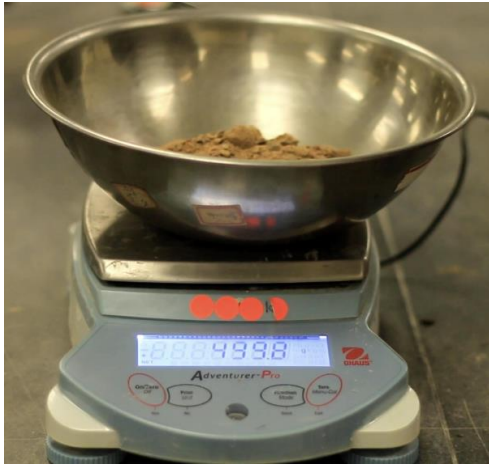
1. Weighing some representative air-dried samples
