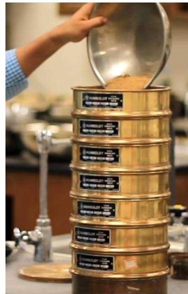
4. Pouring the soil sample at the top of the sieves
