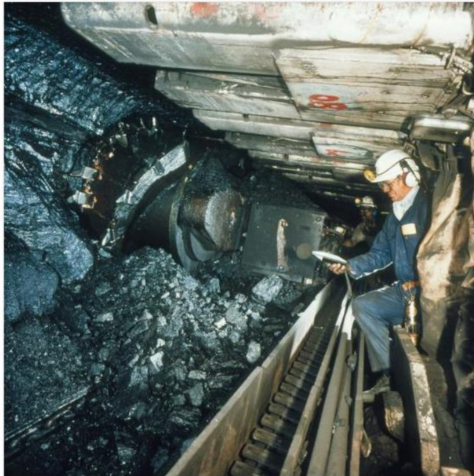
Fig. 1. Measuring noise levels in a coal mine
