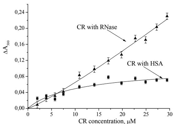
Fig. 6. The isotherm of CR binding to HSA and RNase
